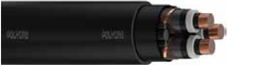
POLYCAB THREE CORE MV AS/NZS 1429.1 1.9/3.3 (3.6) KV (Copper)
